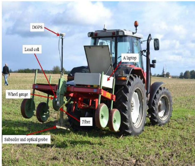
Figure 6. The on-line visible and near infrared (vis-NIR) soil sensor (Mouazen, 2006)
