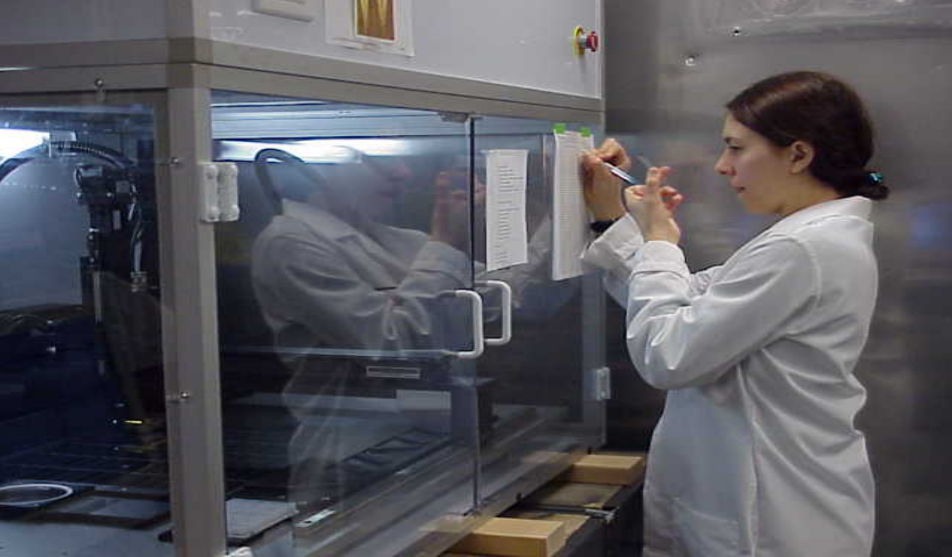
Figure 4. The production of DNA microarrays is automated but it takes a lot of personal attention to details to make sure the robot is performing properly the progress of the robot as it is producing about 100 human DNA chips with 40,000 spots on each chip.
