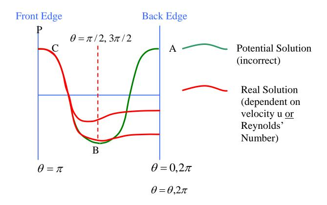
In real flows the fluid is unable to cope with the adverse pressure gradient between  $\theta=3\pi/2$  and  $2\pi$ . This causes the boundary layer to separate from the cylinder, resulting in the development of a low pressure region at the back of the cylinder.
