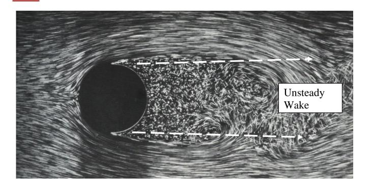
In this case the large pressure differences between the front and the back of the cylinder produces a significant *drag force*. It is usual to define this force in terms of a drag coefficient  $C_{\scriptscriptstyle d}$  such that:
