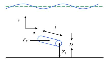
Assuming that the waves are perpendicular to the axis of the cylinder (if not, take the component of the velocity that is). Horizontal force:
