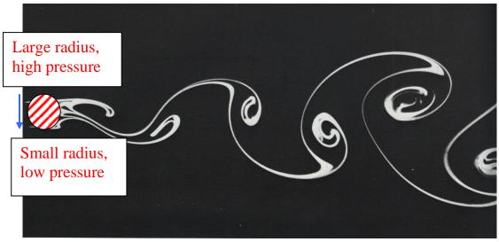
The pressure within a flow depends upon the radius of curvature of the streamlines. It can be shown that a large streamline curvature (small radius) produced smaller pressures. Hence, the above cylinder will tend to move downwards. When the vortex is shed from the opposite side of the cylinder, the pressures will be reverse, and the cylinder will move upwards.
