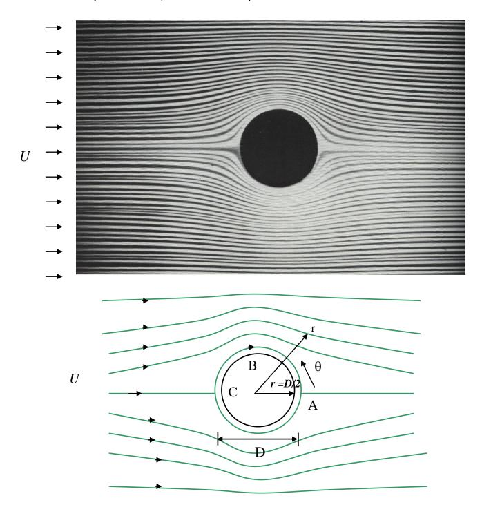
Note: Potential-flow solution is inviscid and irrotational.
