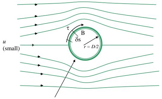
boundary layer – region within which viscosity produces strong shear
