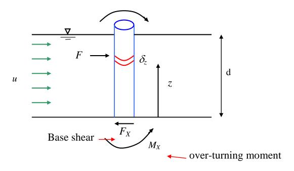
In a steady current  $\frac{du}{dt} = 0$  ... No inertia forces (irrespective of D)
