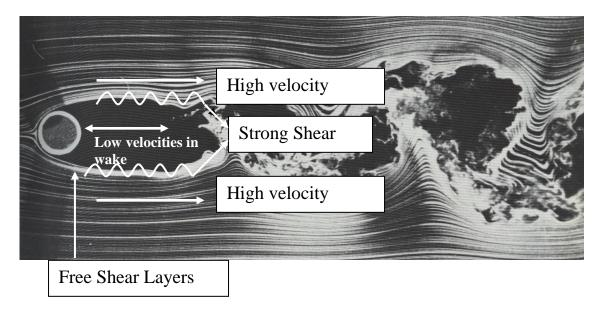
The vorticity within the strongly sheared layers will merge into vortices. These vortices tend to shed from alternate sides of the cylinder leading to the formation of a so-called *Kármán vortex street*.
