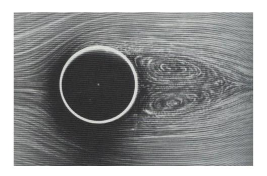
As the velocity increases further, the point of separation moves further around the cylinder and an unsteady wake develops:
