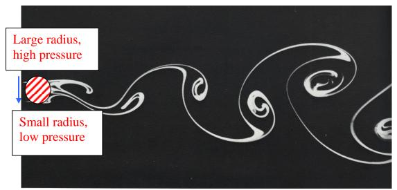
The pressure within a flow depends upon the radius of curvature of the streamlines. It can be shown that a large streamline curvature (small radius) produced smaller pressures. Hence, the above cylinder will tend to move downwards. When the vortex is shed from the opposite side of the cylinder, the pressures will be reverse, and the cylinder will move upwards.
