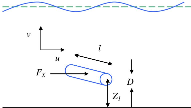
Assuming that the waves are perpendicular to the axis of the cylinder (if not, take the component of the velocity that is).
