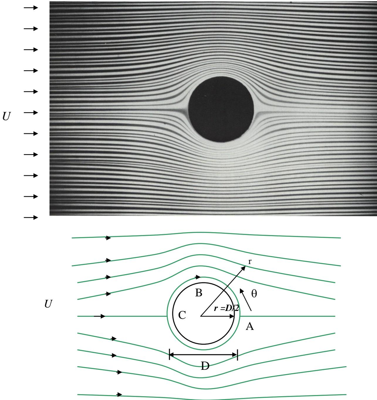
Note: Potential-flow solution is inviscid and irrotational.
