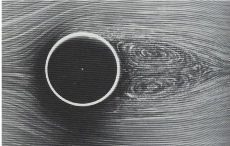
As the velocity increases further, the point of separation moves further around the cylinder and an unsteady wake develops:
