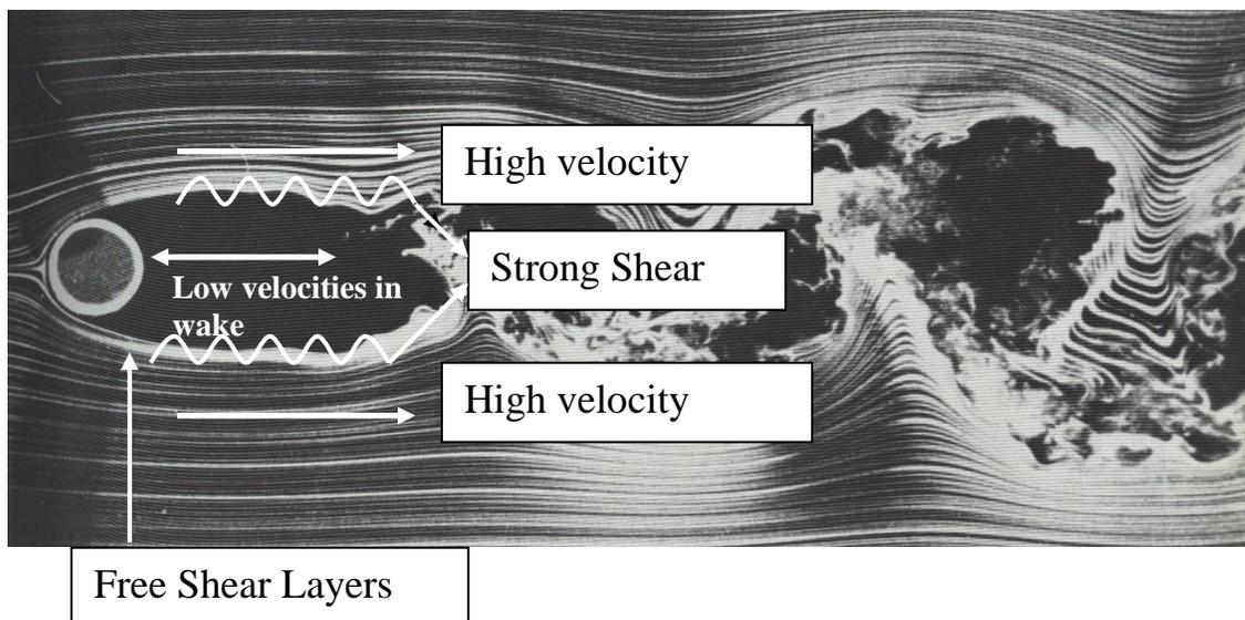
The vorticity within the strongly sheared layers will merge into vortices. These vortices tend to shed from alternate sides of the cylinder leading to the formation of a so-called ***Kármán vortex street***.
