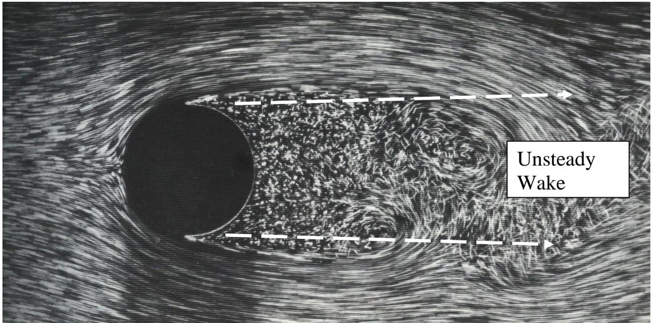
In this case the large pressure differences between the front and the back of the cylinder produces a significant **drag force**. It is usual to define this force in terms of a drag coefficient  $C_d$  such that:
