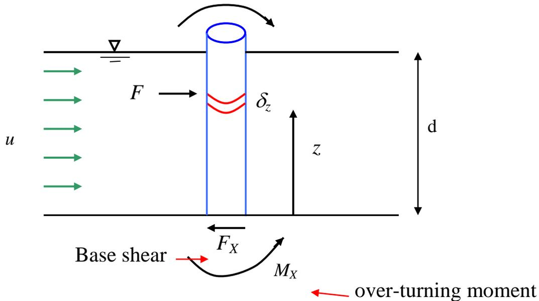
In a steady current  $\frac{du}{dt} = 0 \quad \therefore$  No inertia forces (irrespective of  $D$ )
