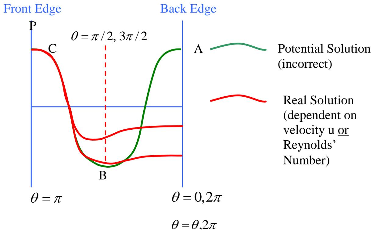
In real flows the fluid is unable to cope with the adverse pressure gradient between  $\theta = 3\pi/2$  and  $2\pi$ . This causes the boundary layer to separate from the cylinder, resulting in the development of a low pressure region at the back of the cylinder.
