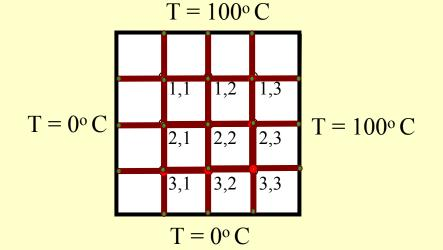
The temperature distribution can be estimated by discretizing the Laplace equation at 9 points and solving the system of linear equations.
