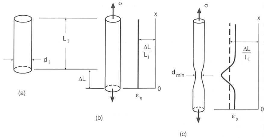
**Figure 4.12** Deformation in a tension test of a ductile metal: (a) unstrained, (b) after uniform elongation, and (c) during necking.
