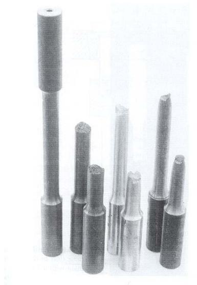
**Figure 4.5** Tensile specimens of metals (left to right): untested specimen with 9 mm diameter test section, and broken specimens of gray cast iron, aluminum alloy 7075-T651, and hot-rolled AISI 1020 steel. (Photo by R. A. Simonds.)
