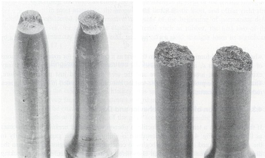
**Figure 4.13** Fractures from tension tests on 9 mm diameter specimens of hot-rolled AISI 1020 steel (left) and gray cast iron (right). (Photos by R. A. Simonds.)
