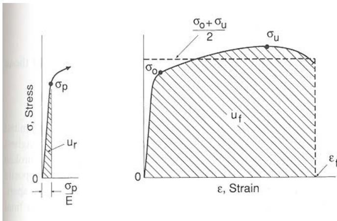
Figure 4.14 Areas under engineering stress-strain curves corresponding to resilience  $u_r$  and tensile toughness  $u_f$ .
