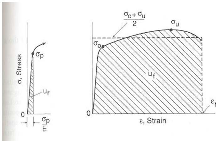
Figure 4.14 Areas under engineering stress-strain curves corresponding to resilience  $u_r$  and tensile toughness  $u_f$ .
