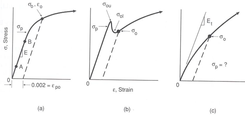
Figure 4.11 Initial portions of stress-strain curves: (a) many metals and alloys, (b) material with yield drop, and (c) material with no linear region.
