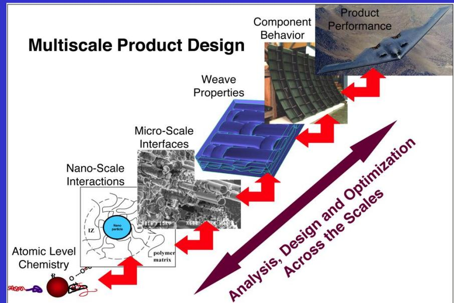
**Multi-scale design** of a composite component of an aircraft (SCOREC, RPI)
