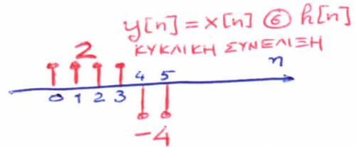
3(E)  $y[n] = ? \text{ με } Y(e^{j\omega}) = X(e^{j\omega}) H(e^{j\omega})$
