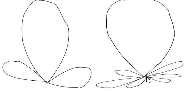
Figure 1: Different shapes of the antenna array radiation diagram as a result of controlling the electric current phases and amplitudes.
