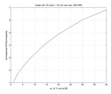
Fig. 10. Optimal sum rate relative to HDR.
