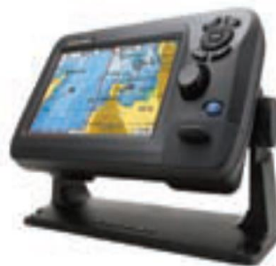
Fig.8. Naval Electronic Instrument displaying and Control Unit for interfacing with: GNSS receivers, satellite compasses, routers etc.
