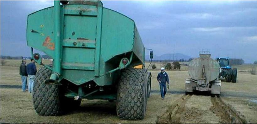
Fig. 3. Excessive rutting caused by narrow high pressure highway tires.
