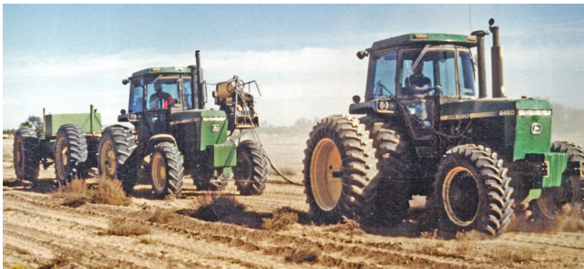
Figure 28. MFWD power hop testing at Firestone Fort Stockton, Texas, Proving Grounds, 1989.
