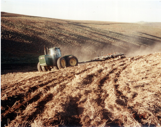
Figure 35. Early experience in controlling 4WD power hop with lower inflation pressures (The Dalles, Oregon, 22 May 1991).
