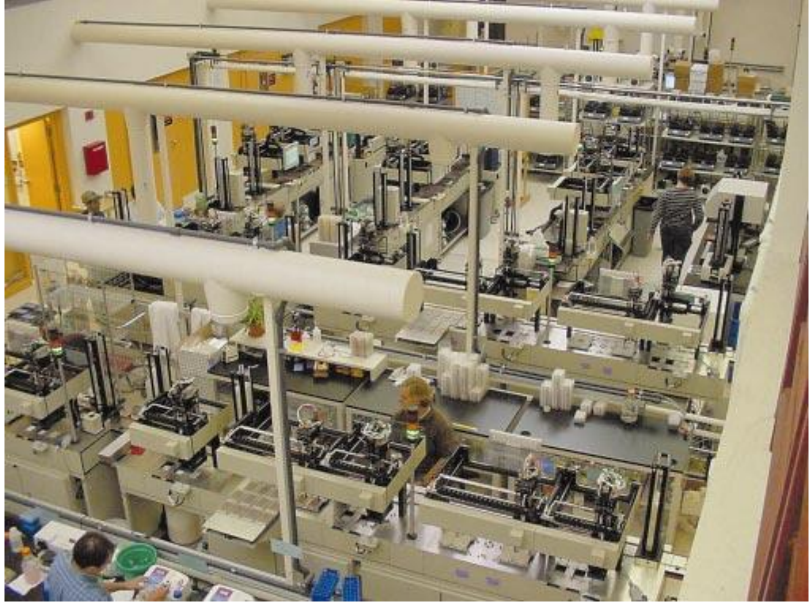
The automated production line for sample preparation at the Whitehead Institute, Center for Genome Research.
