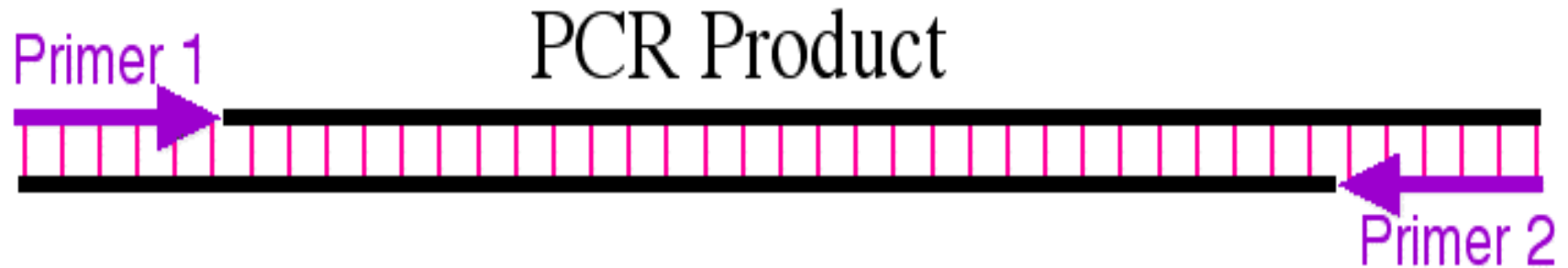
Figure 2. PCR product of interest. The two primers are shown as purple arrows and the base pairing between the two strands is shown in pink.
