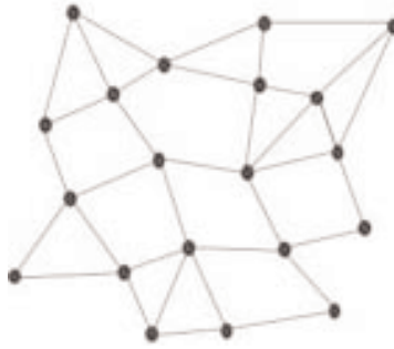
FIGURE 2.1. Baran's feasibility study for RAND determined that a distributed network was the most redundantly connected topology and as such a robust defense against targeted attack. "The enemy could destroy 50, 60, 70 percent of the targets or more and it would still work." 179
