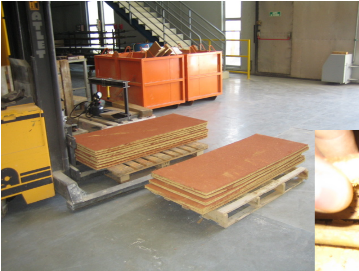
panels of straw and earth
