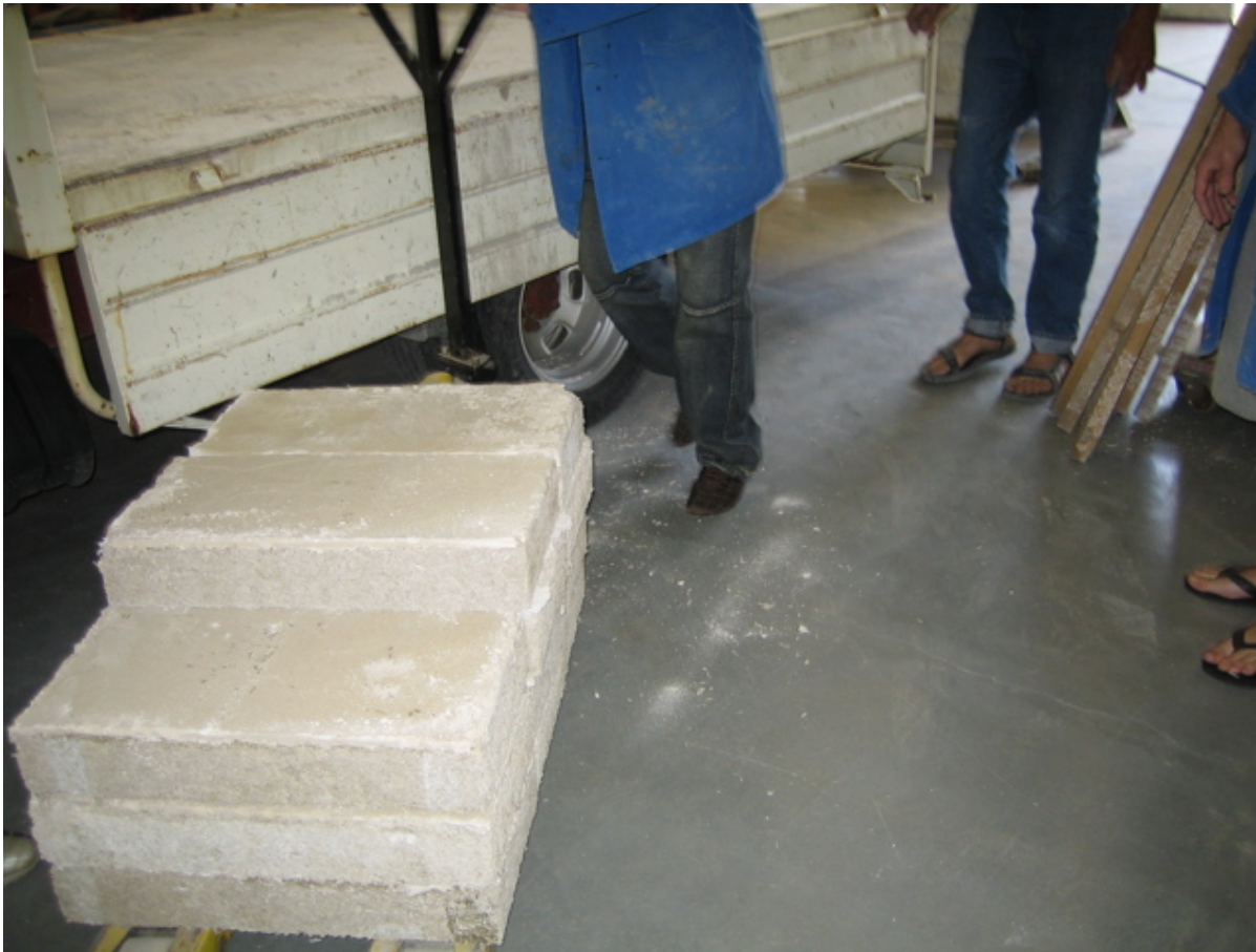
Hemp bricks (+ciment)
