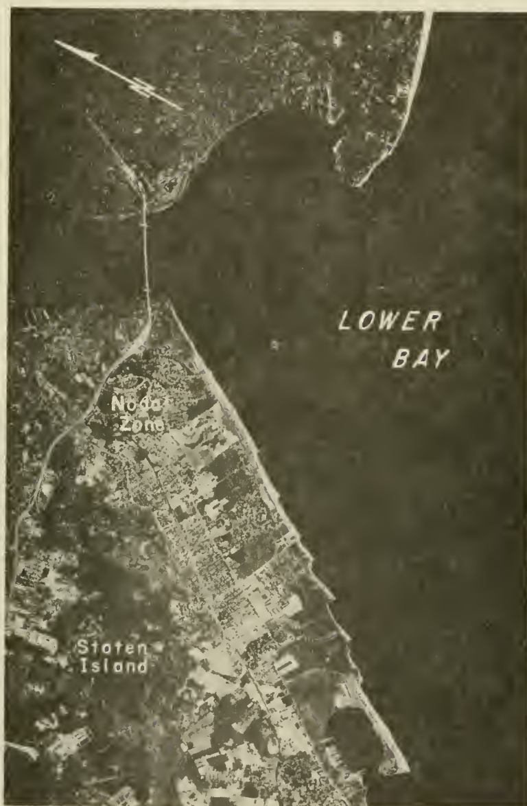
Figure 4-55. Nodal zone of divergence illustrated by sand accumulation at groins, south shore, Staten Island, New York.
