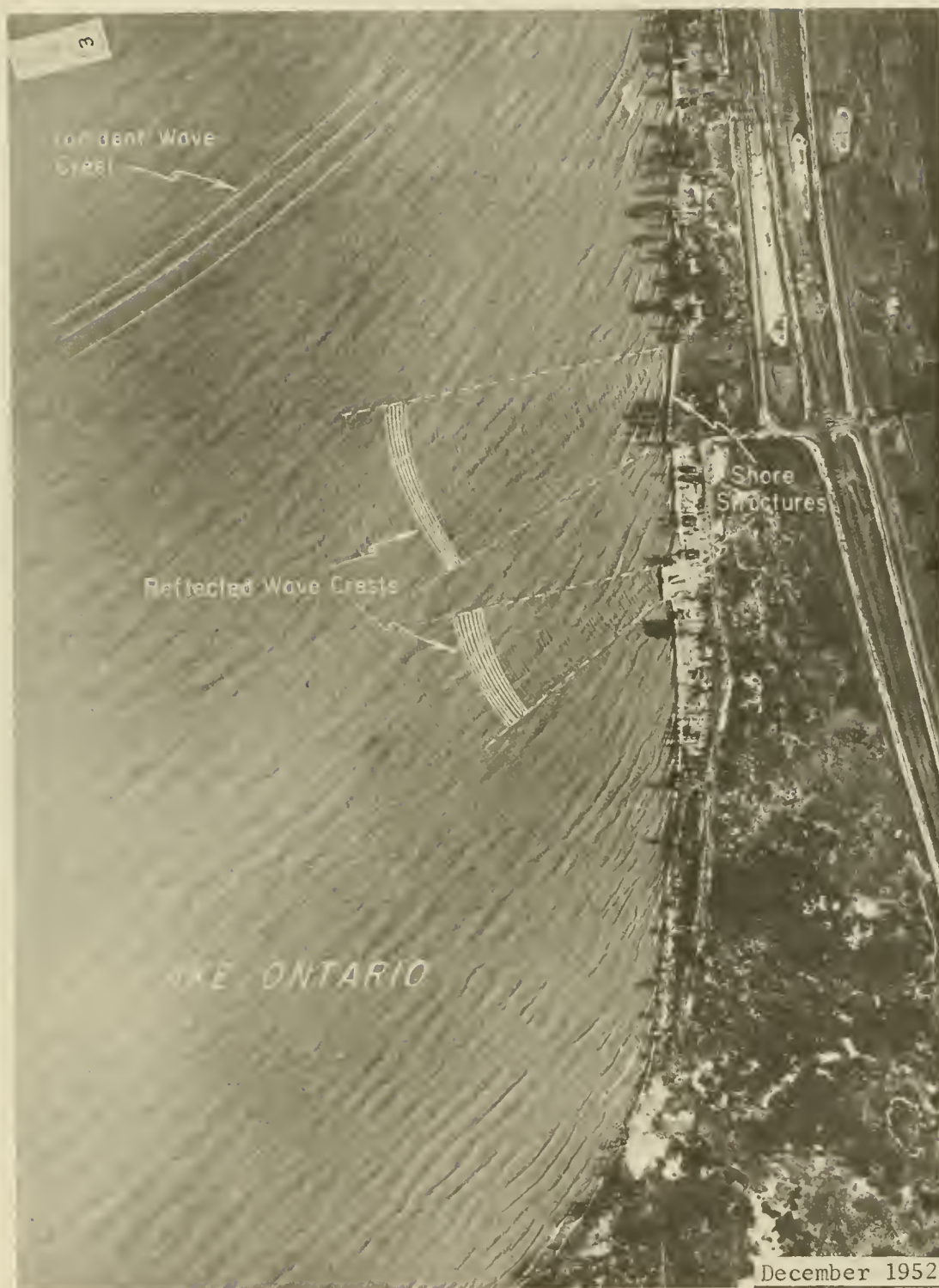
Figure 2-62. Wave reflection at Hamlin Beach, New York.
