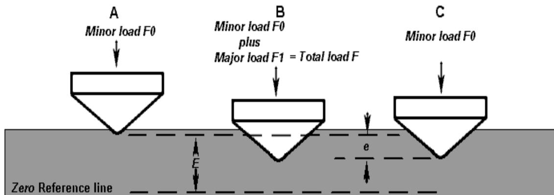
Fig. 1. Rockwell Principle
