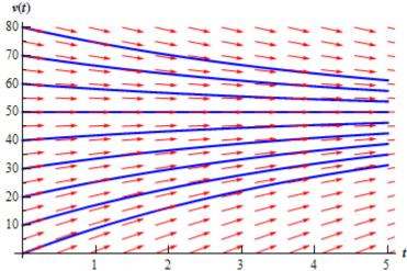
Now, from either the direction field, or the direction field with the solution curves sketched in we can see the behavior of the solution as t increases. For our falling object, it looks like all of the solutions will approach v = 50 as t increases.
