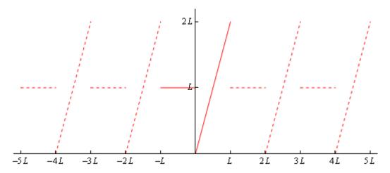
The original function is the solid line in the range  $-L \le x \le L$ . We then got the periodic extension of this by picking this piece up and copying it every interval of length 2L to the right and left of the original graph. This is shown with the two sets of dashed lines to either side of the original graph.
