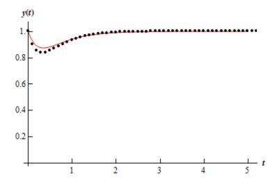
Notice that the approximation is worst where the function is changing rapidly. This should not be too surprising. Recall that we're using tangent lines to get the approximations and so the value of the tangent line at a given *t* will often be significantly different than the function due to the rapidly changing function at that point.
