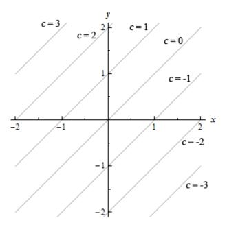
Now, on each of these lines, or isoclines, the derivative will be constant and will have a value of c. On the c=0 isocline the derivative will always have a value of zero and hence the tangents will all be horizontal. On the c=1 isocline the tangents will always have a slope of 1, on the c=-2 isocline the tangents will always have a slope of -2, **etc.** Below is a few tangents put in for each of these isoclines.
