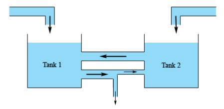
We'll now have two tanks that are interconnected with liquid potentially entering both and with an exit for some of the liquid if we need it (as illustrated by the lower connection). For this situation we're going to make the following assumptions.
