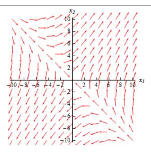
Now all we need to do is sketch in some trajectories. To do this all we need to do is remember that the vectors in the sketch above are tangent to the trajectories. Also the direction of the vectors give the direction of the trajectory as *t* increases so we can show the time dependence of the solution by adding in arrows to the trajectories.
