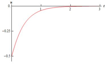
Notice an interesting thing here about the displacement here. Even though we are "over" damped in this case, it actually takes longer for the vibration to die out than in the critical damping case. Sometimes this happens, although it will not always be the case that over damping will allow the vibration to continue longer than the critical damping case.
