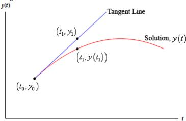
If  $t_I$  is close enough to  $t_0$  then the point  $y_I$  on the tangent line should be fairly close to the actual value of the solution at  $t_I$ , or  $y(t_I)$ . Finding  $y_I$  is easy enough. All we need to do is plug  $t_I$  in the equation for the tangent line.
