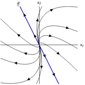
Trajectories in these cases always emerge from (or move into) the origin in a direction that is parallel to the eigenvector. Likewise they will start in one direction before turning around and moving off into the other direction. The directions in which they move are opposite depending on which side of the trajectory corresponding to the eigenvector we are on. Also, as the trajectories move away from the origin it should start becoming parallel to the trajectory corresponding to the eigenvector.
