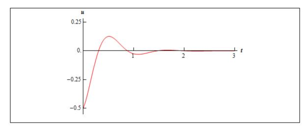
In this case we finally got what we usually consider to be a true vibration. In fact that is the point of critical damping. As we increase the damping coefficient, the critical damping coefficient will be the first one in which a true oscillation in the displacement will not occur. For all values of the damping coefficient larger than this (*i.e.* over damping) we will also not see a true oscillation in the displacement.
