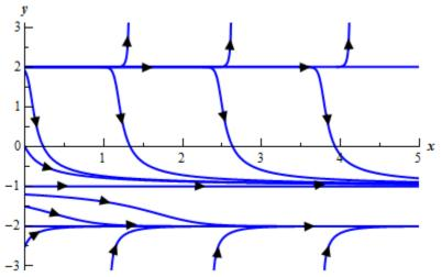
From this it is clear (hopefully) that y = 2 is an unstable equilibrium solution and y = -2 is an asymptotically stable equilibrium solution. However, y = -1 behaves differently from either of these two. Solutions that start above it move towards y = -1 while solutions that start below y = -1 move away as t increases.
