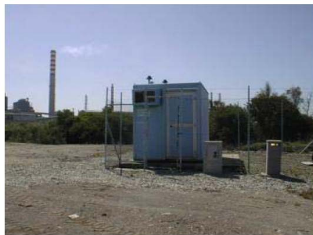
Figure 2 Example of an industrial station. The measurement station Portoscuso – Rio su Cannoni (35) of the monitoring network of the Province of Cagliari, Italy. Photo © Provincia di Cagliari, Italy.
