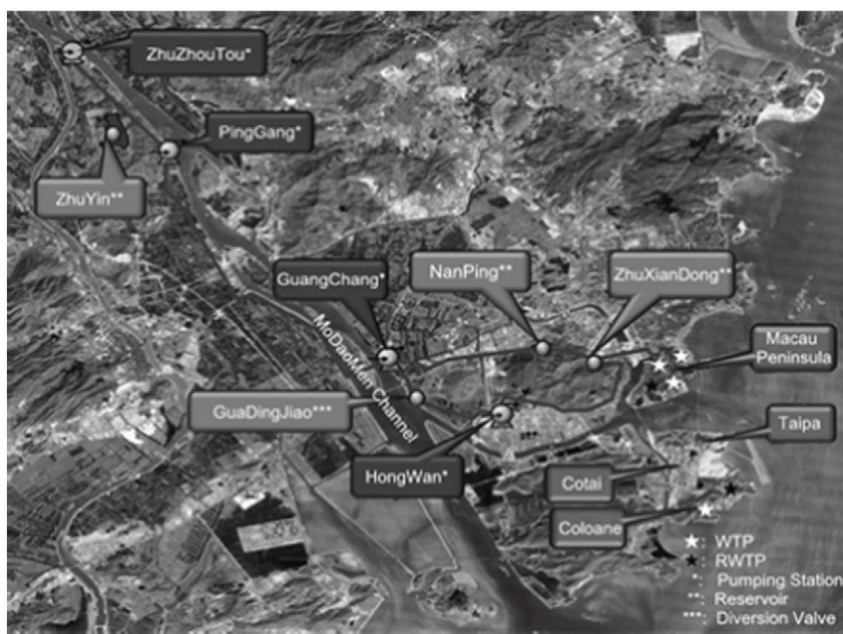
Fig. 1 – Raw water supply system of Macau.
