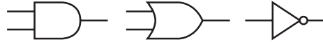
FIGURE B.2.1 Standard drawing for an AND gate, OR gate, and an inverter, shown from left to right. The signals to the left of each symbol are the inputs, while the output appears on the right. The AND and OR gates both have two inputs. Inverters have a single input.
