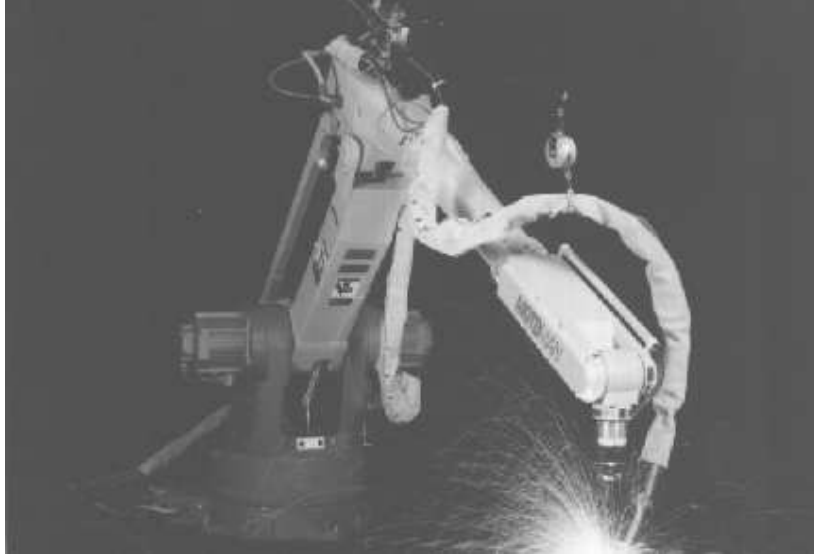
Figure 6.4: The Motoman K10MSB robot performing an arc welding task. (Photograph courtesy of Motoman)
