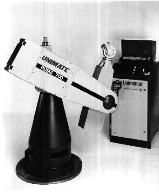
Figure 1.3: The Unimation PUMA (Programmable Universal Manipulator for Assembly). (Courtesy of Stäubli Unimation, Inc.)
