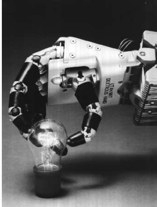
Figure 1.8: The Utah/MIT hand. (Photo courtesy of Sarcos, Inc.)
