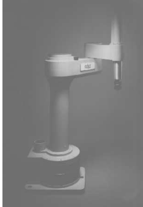
Figure 1.4: The AdeptOne robot. (Courtesy of Adept Technology, Inc.)
