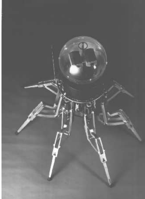
Figure 1.6: The Odex I six-legged walking robot. (Photo courtesy of Odetics, Inc.)
