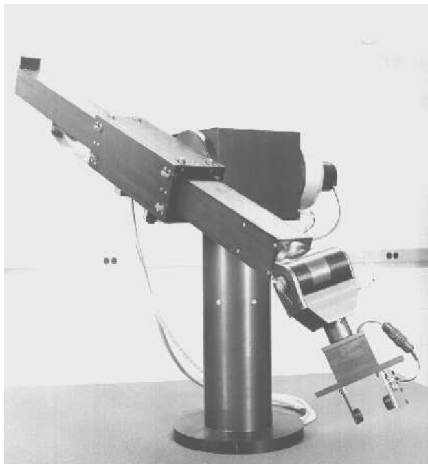
Figure 1.1: The Stanford manipulator. (Courtesy of the Coordinated Science Laboratory, University of Illinois at Urbana-Champaign)
