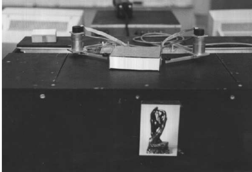
Figure 1.10: Styx, a two-fingered planar hand built at UC Berkeley in 1988.
