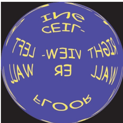
Color Plate 7. (Figure V.10, page 138.) An environment map mapped into a sphere projection. This is the kind of environment map supported by OpenGL. The scene is the same as is shown in Figure V.11. Note that the front wall has the most fidelity and the back wall the least. For this reason, spherical environment maps are best used when the view direction is close to the direction used to create the environment map.
