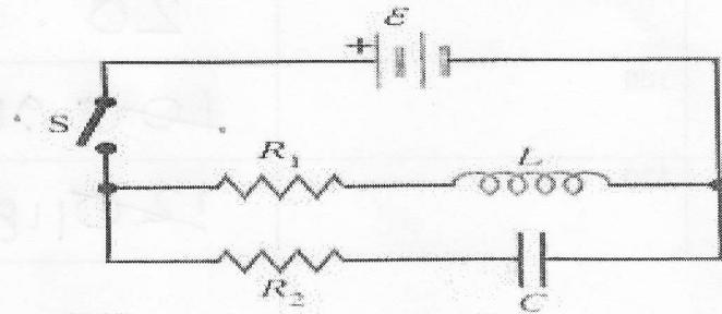
όπου  $\epsilon = 60V$ ,  $L = 10H$ ,  $C = 20\mu F$ ,  $R_1 = 25\Omega$ ,  $R_2 = 5k\Omega$ .
