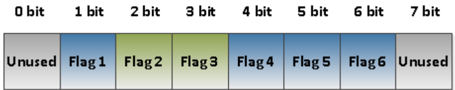
Figure 4.4.2 – Description of the Flags Field in STUXNET_CC_MESSAGE Structure
