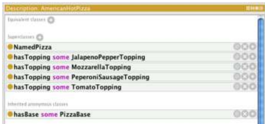
Figure 4.37: The Class Description View displaying the description for AmericanHotPizza
