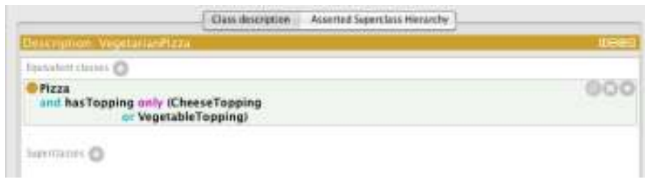
Figure 4.50: The Class Description View Displaying the Definition of VegetarianPizza (Using Necessary and Sufficient Conditions)
